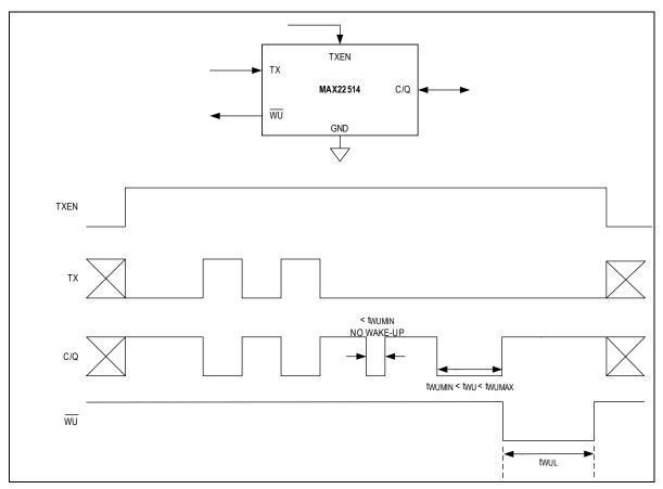
Figure 5. Wake-Up Detection Timing
