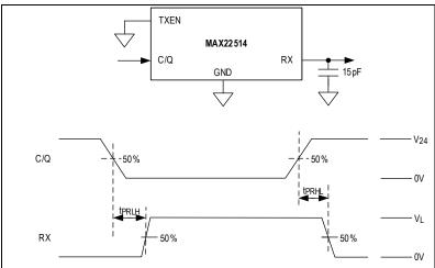
Figure 4. C/Q Receiver Timing
