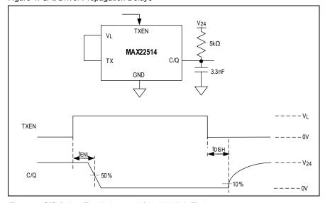
Figure 2. C/Q Driver Enable Low and Disable High Timing
