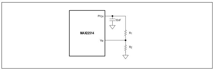
Figure 8. VM input used to monitor the PV24 supply
