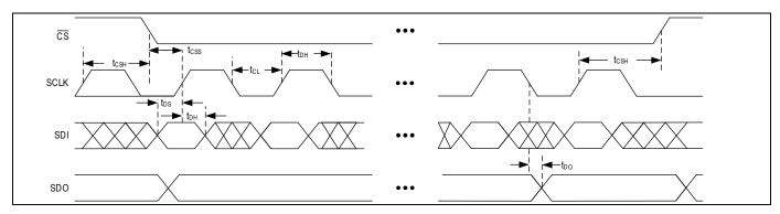
Figure 7. SPI Timing Diagram
