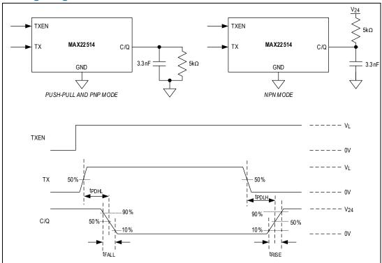
Figure 1. C/Q Driver Propagation Delays
