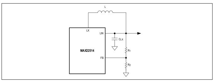
Figure 9. Setting the DC-DC Output Voltage
