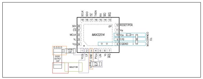
Figure 12. Sample Grounding Scheme (TQFN Package)
